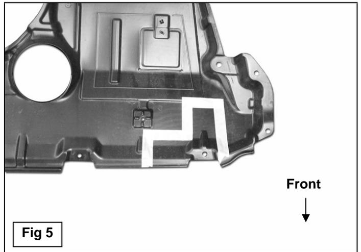
Hold the plastic splash guard up to the bottom of the brackets. Trace location of brackets onto the inside of the splash guard. Picture used for example only
