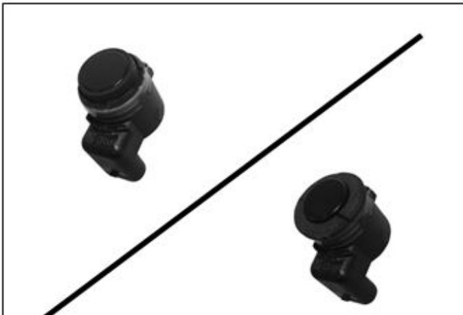
(Fig 10) Remove OE sensor washer and place the provided Foam Washer onto the front of the sensor
