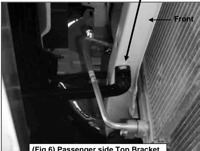
(Fig 6) Passenger side Top Bracket installation pictured from below
