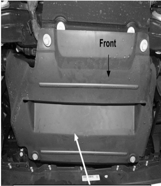
**Fig4B: Remove hardware attaching plastic fill panel to inner fender**
