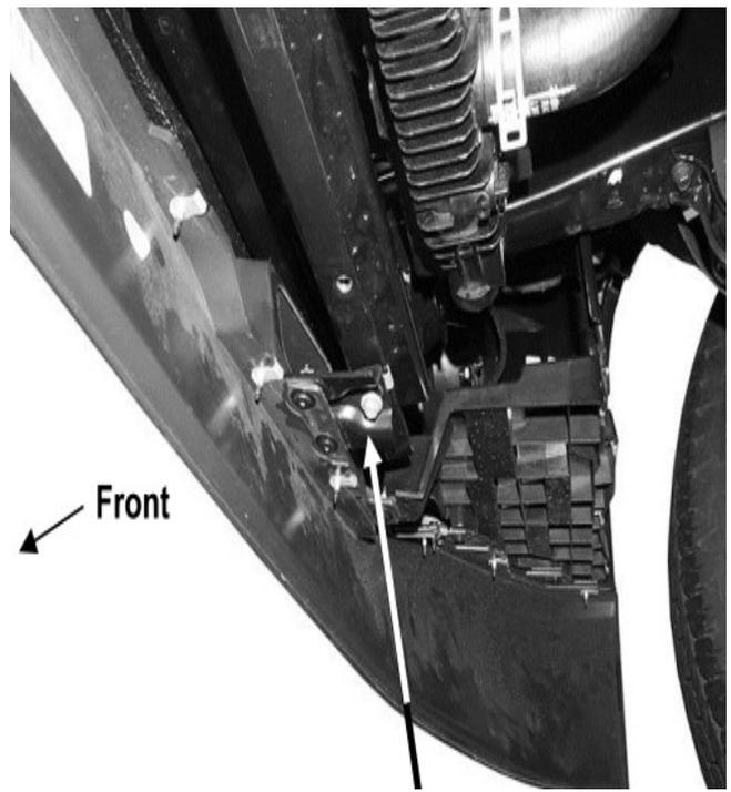
**Fig4C: Remove hardware attaching fender liner to bumper cover**
