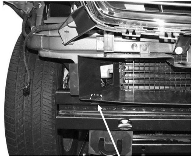
**Fig8: Air deflector cut to clear Top Bracket
